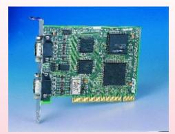
PCI 2 Port RS422/485 PCI card with Baud Rates up to 15,000,000 baud (15 MegaBaud)
